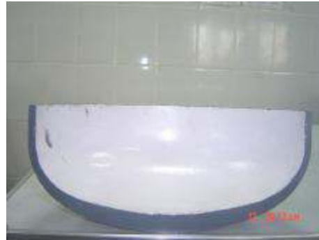
Cut section of type 1 CNG Cylinder bottom
