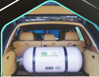
COMPRESSED NATURAL GAS CYLINDERS
