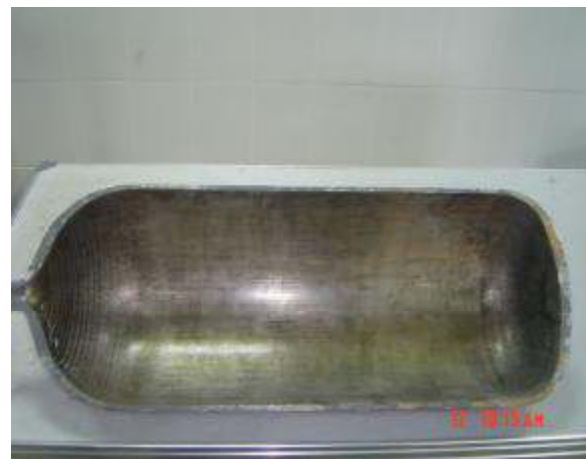
Cut Section of type 1 CNG Cylinder
