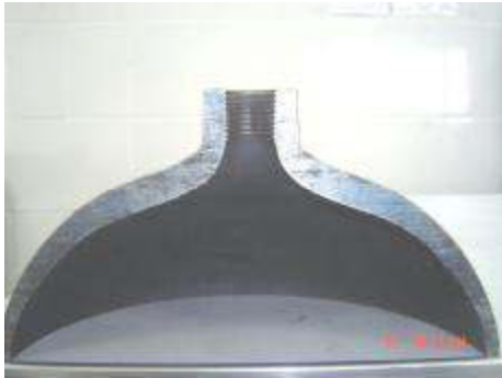
Cut Section of Type 1 CNG Cylinder Neck
